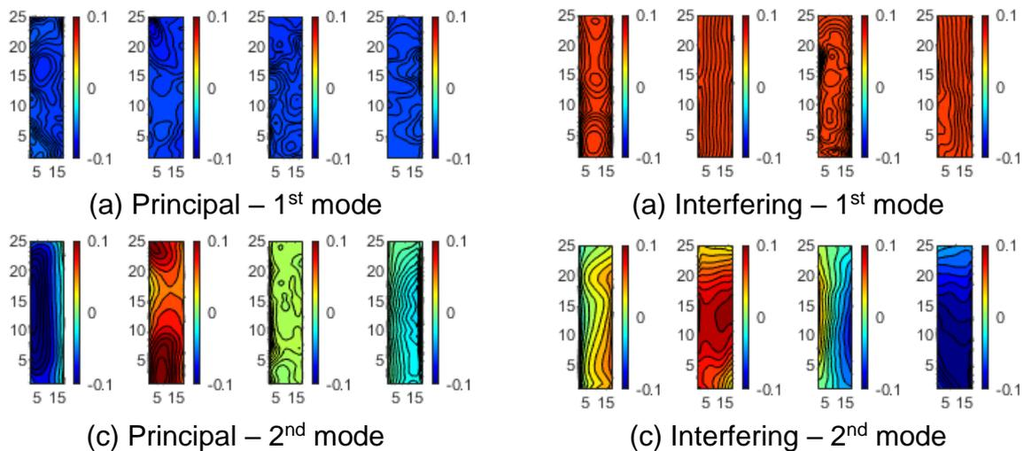
Fig. 3 POD mode shape of fluctuating wind pressure on building
