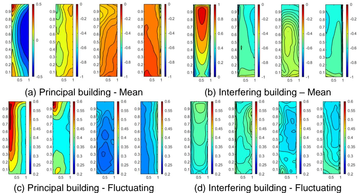
Fig. 1 Mean and fluctuating wind pressures on building
